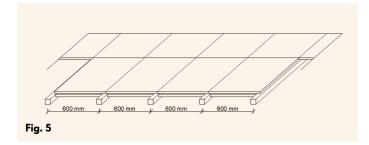
*VMG Lignum Board* | *Floor* are nailed or screwed. In service class 1, galvanize steel or stainless steel and in service class 2 - hot galvanized steel or stainless steel fasteners must be used. The minimum length of fasteners must be at least 50 mm or twice the thickness of the panel, whichever is the longest. For nails, the minimum diameter is 0.16 times the thickness of the panel; and 0.2 times the thickness of the the panel for screws. Minimal nails 3.0/50 mm, screws 3.6/50 mm.
