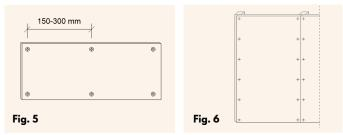
*VMG Lignum Board* | *Wall T&G2* must be supported on 2 sides (Fig. 6). This support should be 18 mm at least (Fig. 8)
