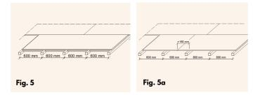
*VMG Lignum Board* | *Floor* are nailed or screwed. In service class 1, galvanize steel or stainless steel and in service class 2 - hot galvanized steel or stainless steel fasteners must be used. The minimum length of fasteners must be at least 50 mm or twice the thickness of the panel, whichever is the longest. For nails, the minimum diameter is 0.16 times the thickness of the panel; and 0.2 times the thickness of the the panel for screws. Minimal nails 3.0/50 mm, screws 3.6/50 mm.
