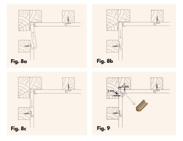
For external corners the first board should be cut 3mm in length, the final board – 10 mm. Edge of the board must be chamfer. The board marked with number 1 is installed first and then board marked with number 2.
