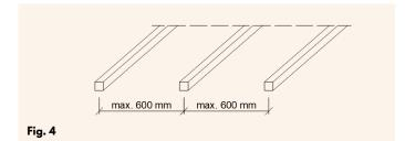
*VMG Lignum Board* | *Floor* should always be perpendicular to the direction of the beams (Fig. 5). All short panel edges must be supported. *VMG Lignum Board* | *Floor* must span at least 600 mm gaps, and connection must always be formed on the centre-line of a beam. In this case minimum distance from beam to joint should be 160 mm. If the short joints end up between the same pair of beams, the distance between the short joints must be the minimum 360 mm.
